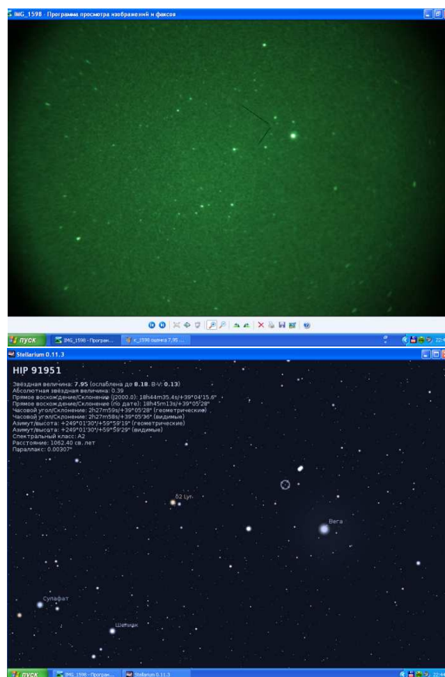
Figure 3 – Estimation of the setup limiting magnitude by stars. Photo of the Lyra constellation via our setup. Selected with the lines star is HIP 91951 (+8 m ). Half of the photo field of view in the STELLARIUM program.
