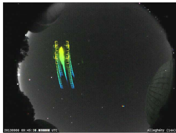
Figure 11 – Stacked video frames of a poorly tracked meteor. In each frame, ASGARD marks the meteor's location by drawing the corners of a square around it. One can see that when the meteor is at its brightest, these markers exhibit some left-right and up-down jitter, as the tracking jumps ahead to illuminated clouds in front of the meteor and then falls behind it to lock on the illuminated trail.
