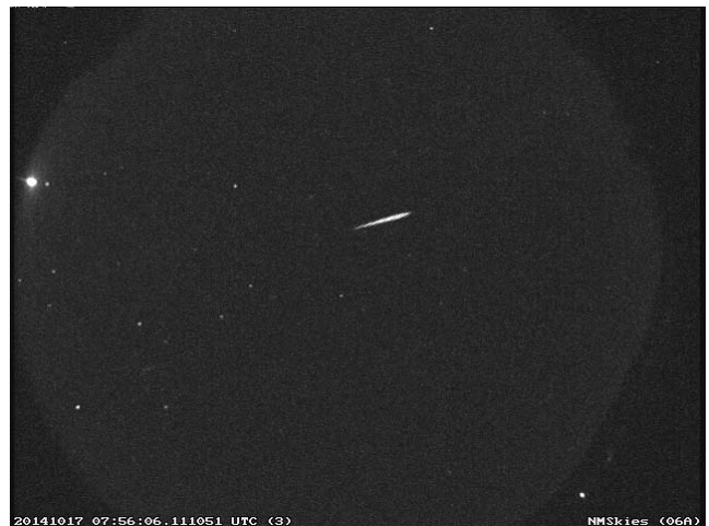
Figure 2 – Composite image of an Orionid meteor detected by the NASA All Sky Fireball Network on 2014 October 17. This image illustrates the basic characteristics of our meteor imagery: black-and-white images, a large field of view that encompasses most of the horizon, and the ability to detect a few stars (the constellation Orion is easily seen in the lower left quadrant). Images are oriented with north at the top and west to the right.
